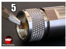
Fasten together the connector and component A, until it will be pressed against the connector body. Inside, the rubber component C (pic. 1) will expand, granting optimal sealing against moisture and a perfect contact to ground.
