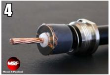
Cut and remove the tape and dieletric for a lenght as shown in the picture.(20mm)
